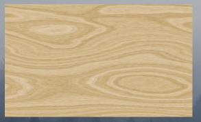
Superpower: Plywood is an engineered wood product where wood is glued together to make a flat sheet. It is versatile, very stable, and has high impact resistance. It can have a natural wood grain look with a veneer layer
