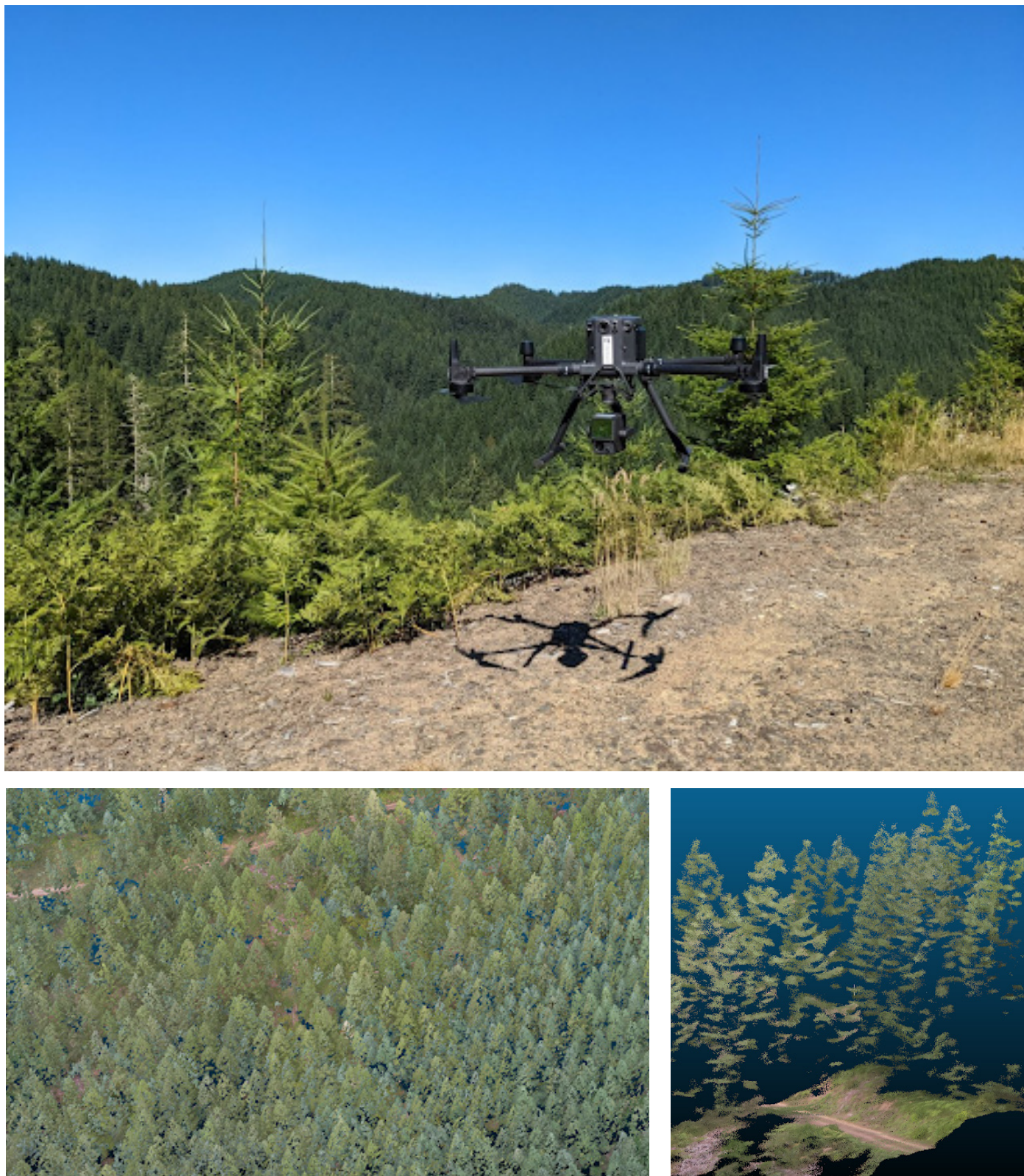
Figure 10.1. Return to home of a UAS LiDAR flight on upper Lost Creek (top). Resulted point clouds at the perspective view of an upper side of the ridge (bottom left) and zoom in around the road (bottom right).
