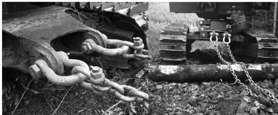
Figure 4. Left. A custom designed hitch for a remotely powered, tethered feller-buncher. Right. Protective chain attachment to hitch point.
