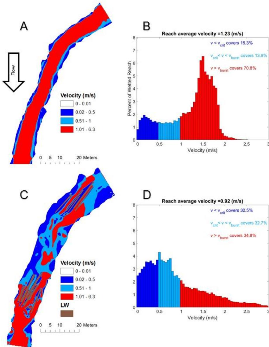
Figure 2: Spatial and frequency distributions of velocity at bankfull discharge before (A and B) and after (C and D) the addition of large wood (LW) in Mill Creek. Colors correspond to thresholds of velocity relevant to the ability of juvenile Coho Salmon to maintain position in the stream (dark blue  $v < v_{crit}$  where  $v_{crit} = 0.5$  m/s, light blue  $v_{crit} < v < v_{burst}$  where  $v_{burst} = 1$  m/s, and red  $v > v_{burst}$ ).
