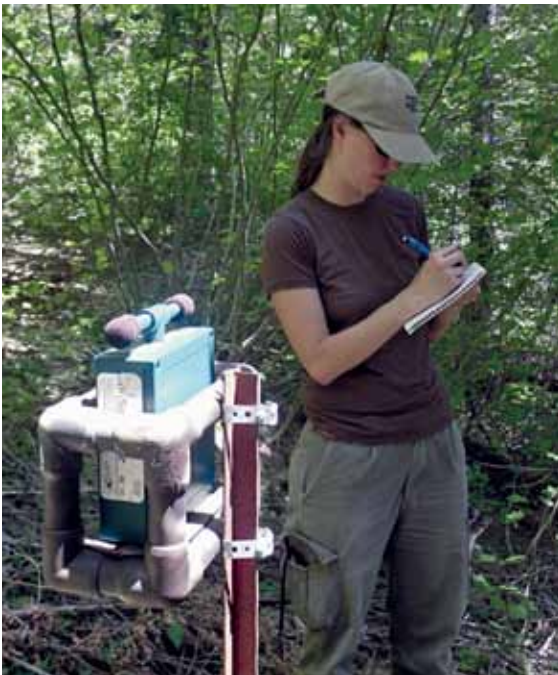
Researcher Sarah Hadley (PhD student, FES) is using this instrument to monitor bird sounds in the forest. This technology is far more effective than any available before. Photo credit: Forrest Briggs.
