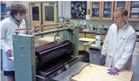
(Top) Thor Dodson (RM) making a wood fiber composite with a hot press; Dodson and Elijah Wilson (RM) pressing LVL in the composites lab in Richardson. Photo credit: Logan Bernart.
