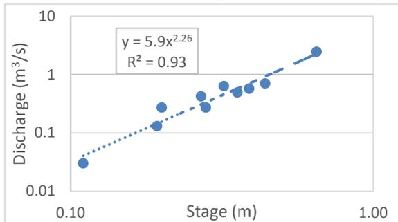
Figure 3: Rating curve for site 2. Given here as an example.
