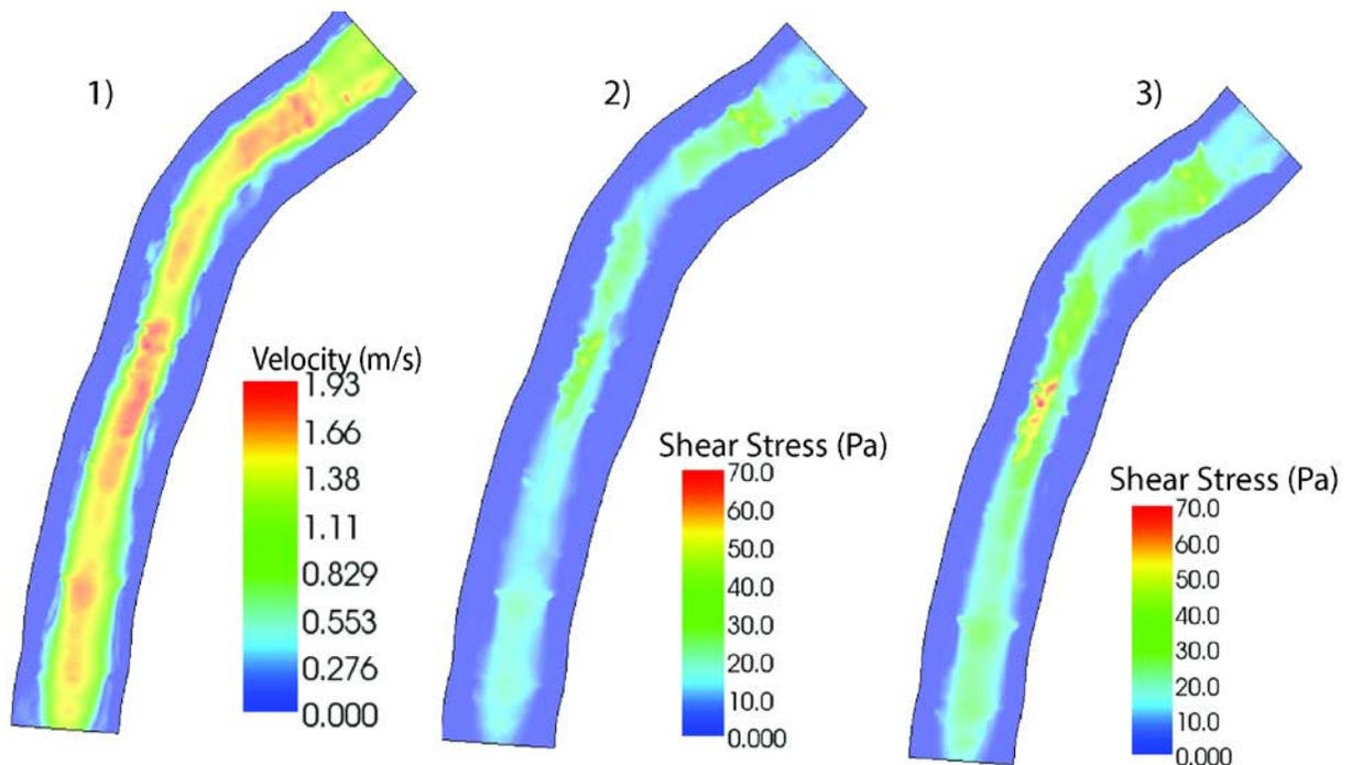
Figure 5: Example of modeled distributions of velocity and shear stress at Site 1. 1) Modeled velocity distribution at bankfull flow ( $Q_{bf}$ ); 2) shear stress distribution at  $0.45Q_{bf}$ ; and 3) shear stress distributions at  $Q_{bf}$ .
