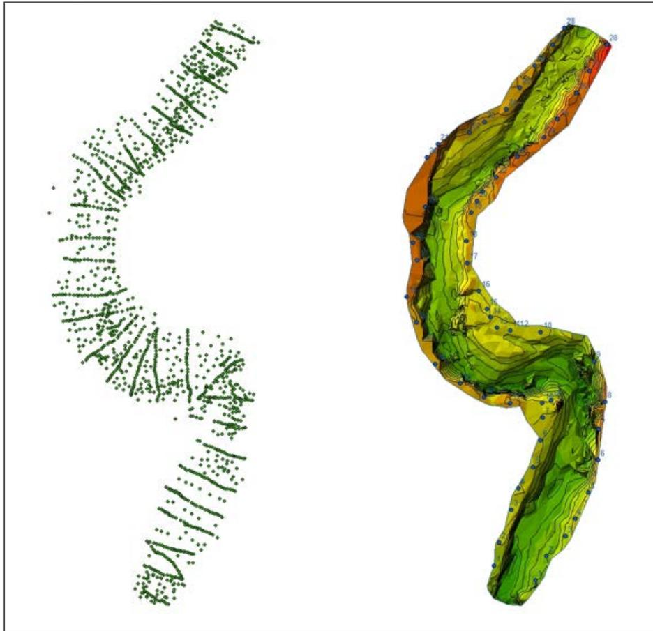
Figure 2: Site 3 survey points and interpolated channel geometry
