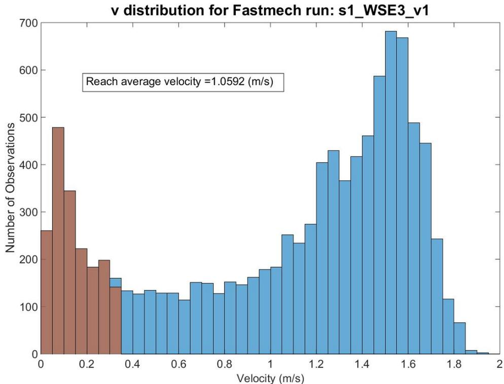
Figure 6: Modeled distribution of velocity for site 1 during a flow event of  $8.6 \text{ m}^3/\text{s}$  (90% of  $Q_{bf}$ )
