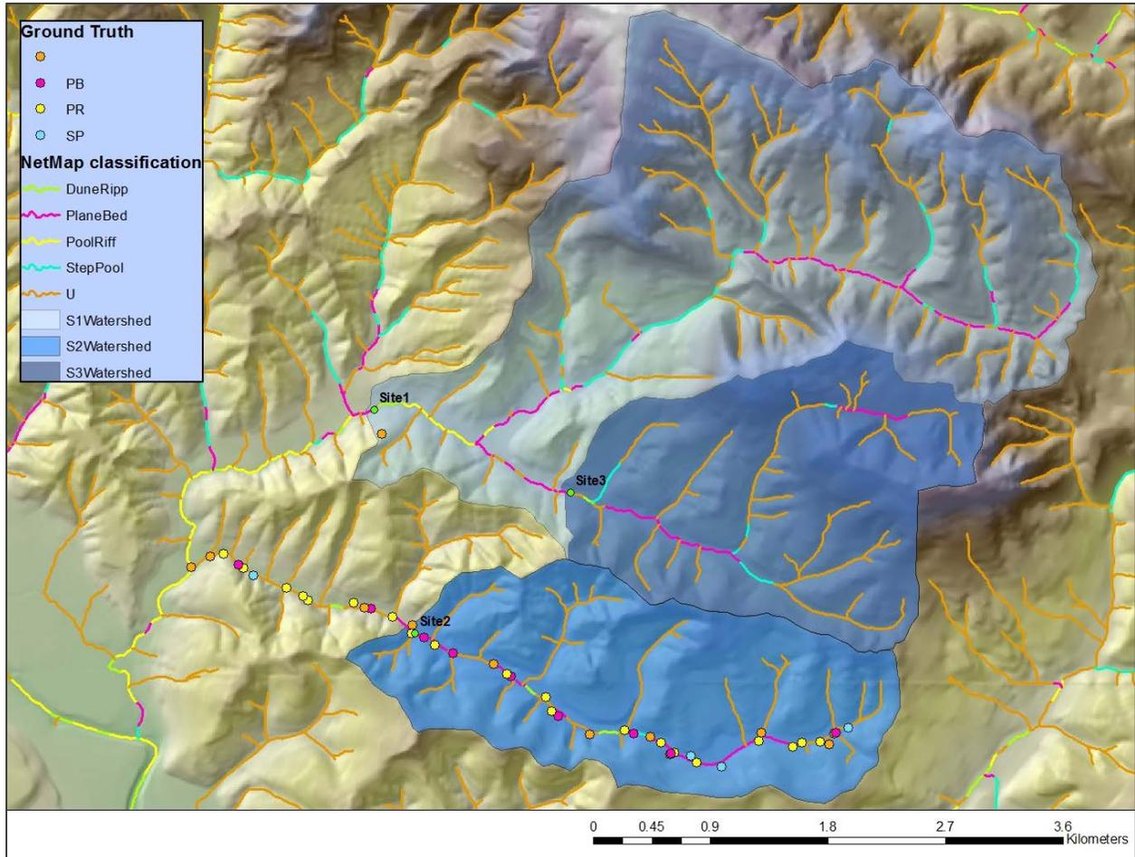
Figure 7 Channel type based on slope, and field observations
