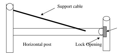
The lock opening in the small post is a favorite place for wasps and hornets to build nests. In addition, vandals have been known to place broken glass and other objects inside these openings. *NEVER place your hands inside to open a lock without first looking inside*.
